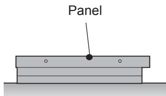
If there is not a cushion available, ensure the floor is clean and then lay the product down carefully with the panel facing either upward or downward. At this time, be careful for objects not to fall on the panel.
