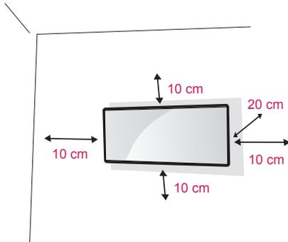
Install the monitor at least 10 cm away from the wall and leave about 10 cm of space at each side of the monitor to ensure sufficient ventilation. Use the wall mount plate and screws that comply with the VESA standard.
