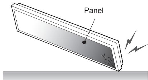
If the product is tilted onto the edge of the panel, the panel may be damaged.
