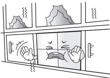
Do not install the product in a place with no ventilation (e.g., on a bookshelf or in a closet) or on a carpet or cushion. If there is no other option but to mount the product on the wall, make sure that sufficient ventilation is provided before installation.
