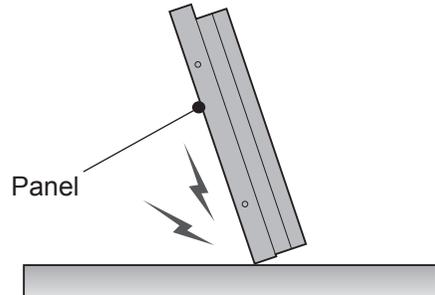
If the product is tilted onto the bezel, the bottom of the panel may be damaged.
