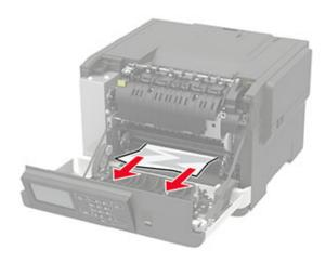
**3** Open the fuser access door, and then remove the jammed paper.
