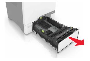
**2** Remove the separator bracket.
