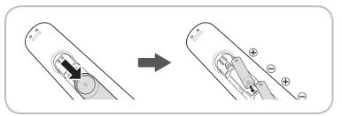
After you have installed the batteries, use a screwdriver to screw in the screw that holds the battery cover closed.
