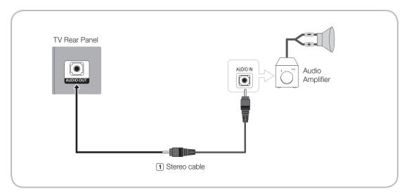
1. Connect the AUDIO OUT port of the TV to the Audio In port of an audio amplifier with a stereo cable. (Stereo cable not provide)
