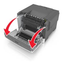
**3** Slide the release latch on the right side of the printer, and then open the top door.
