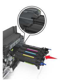
15 Gently, but firmly push the blue levers down until the imaging kit fits into place.
