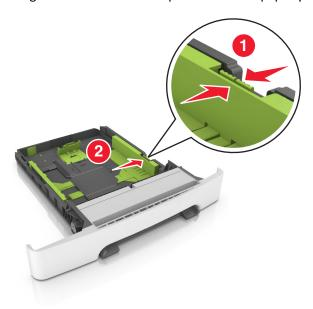
**3** Squeeze, and then slide the length guide tab to the correct position for the paper you are loading.
