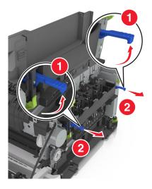
Press down the blue lever, and then grasp the green handles on the sides to pull out the imaging kit.
