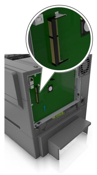
**Warning—Potential Damage:** Controller board electronic components are easily damaged by static electricity. Touch something metal on the printer before touching any controller board electronic components or connectors.
