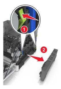
Lift the blue levers on the imaging kit, and then pull the imaging kit until it stops.
