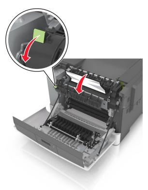
**3** Hold down the fuser cover, and then remove the jammed paper.
