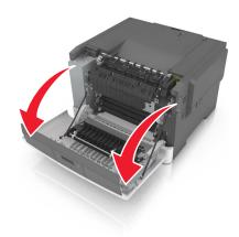
**2** Pull the green lever to open the fuser cover.
