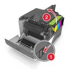
3 Remove the toner cartridges by lifting the handles, and then gently pulling them away from the imaging kit.
