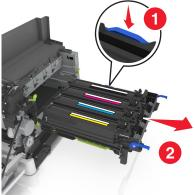
**8** Remove the used developer unit.
