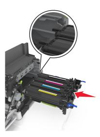
13 Gently, but firmly push the blue levers down until the imaging kit fits into place.
