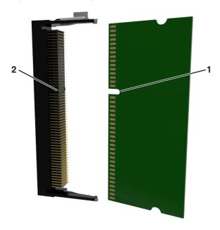
**7** Push the memory card straight into the connector, and then push it into the controller board wall until it *clicks* into place.
