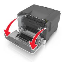
**2** Slide the release latch on the right side of the printer, and then open the top door.
