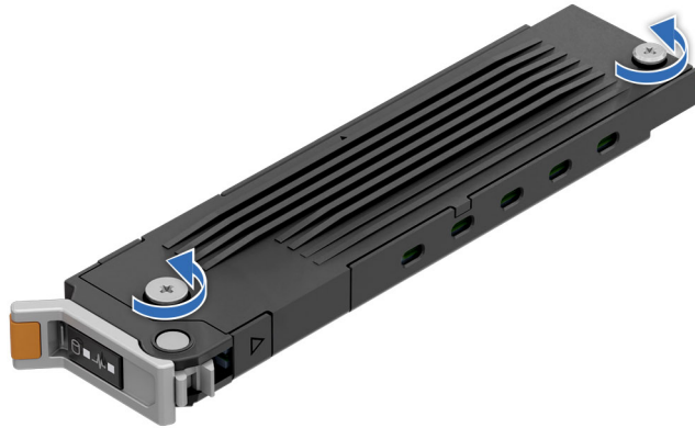
Figure 166. Loosen the top cover captive screws
