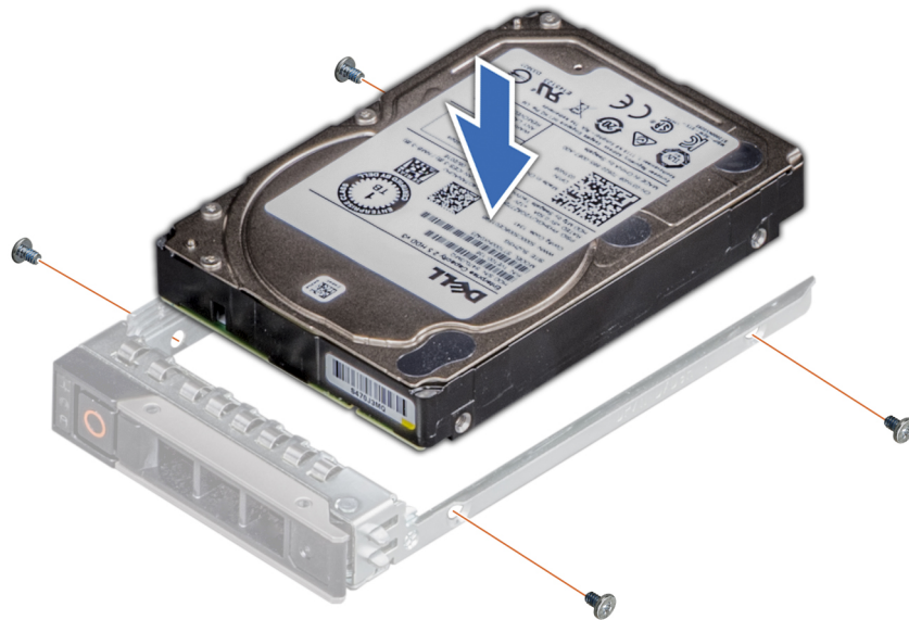
Figure 62. Installing a drive into the drive carrier
