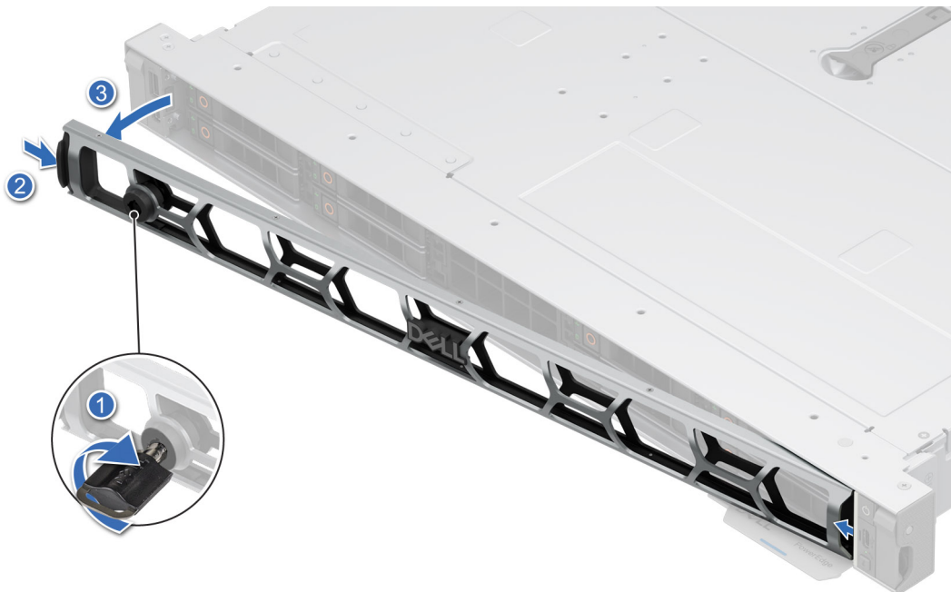
Figure 36. Removing the front bezel
