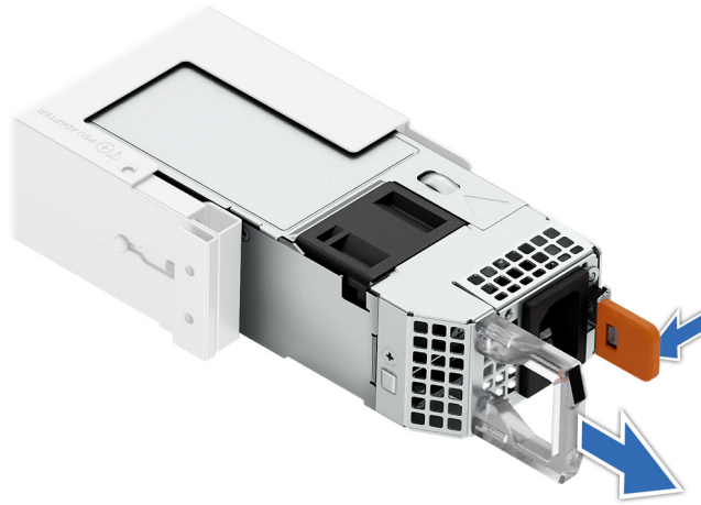
Figure 224. Removing a power supply unit
