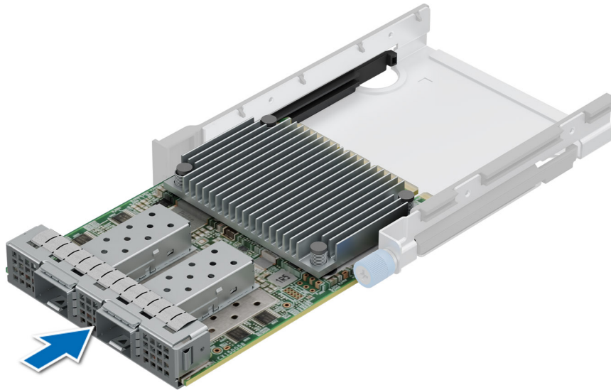
Figure 202. Installing the OCP NIC card into the OCP NIC card tray
