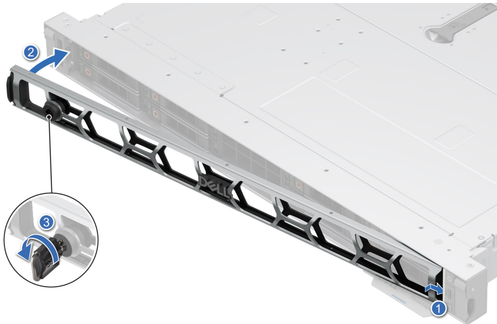
Figure 37. Installing the front bezel
